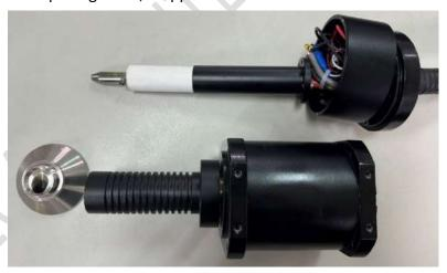
(6) Loosen the screw on the electrode, turn the electrode counterclockwise to remove it from the ceramic thread, and after replacing it with a new electrode, tighten the screw to ensure proper contact.
